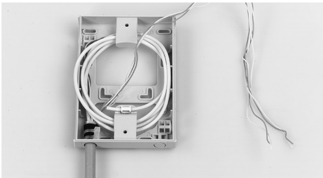
1.2.20 Hybrid cable: storage of loose tube, using copper wires only. Max. 1.4 m of loose tube storage (diam. 2.7 mm).
