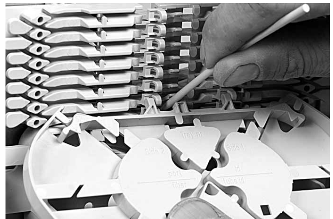
6.5 To remove the tray put the fiber guiding pin between lip on wraparound groove plate and tray and move lateral towards S1.
