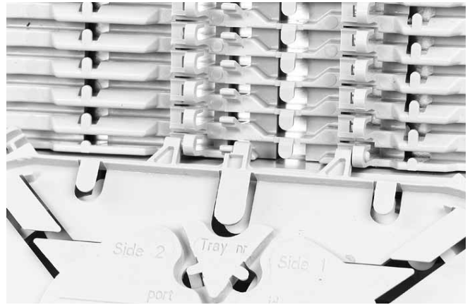
6.4 Place a tray in the wraparound groove plate; do this by pushing the lip on the groove plate (lowest possible position) slightly down with the tray and move the tray lateral into the hinge-cavities of the groove plate. To snap the High Capacity Single Element tray (HCSE) in the W/a single fiber groove plate leave always one hinge facility open between Fasblock or previous tray and the HCSE-tray.
