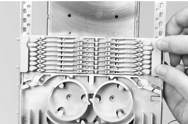
6.3 To remove push the two snapfits at S2 UMS-profile and slide the wraparound plate towards S1 UMS-profile.
