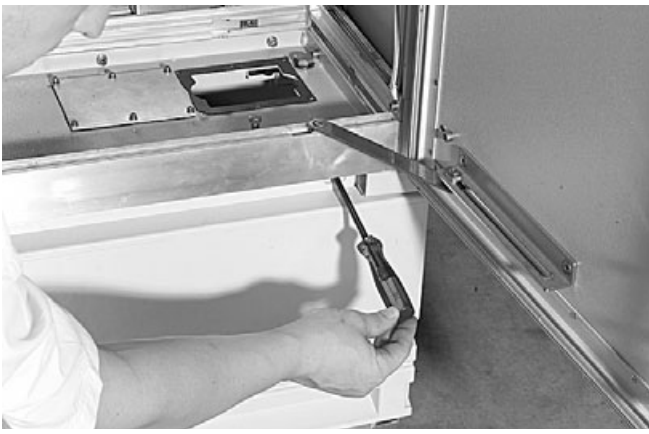
10.2.9 Place the cover on the pedestal.
