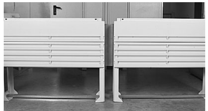
9.1.10 Align the two pedestals and tighten the nuts of the second pedestal.
