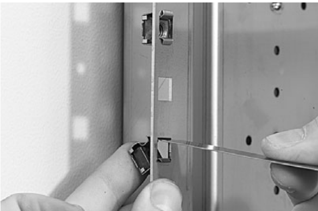
4.2.1 Mount the cage nuts at the correct locations, using the cage nut tool.
