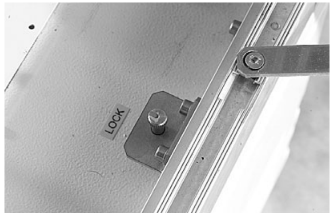
9.2.11 Lock the protection plate
