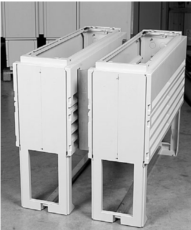
10.1.8 Align the two pedestals, and tighten the nuts of the second pedestal (20-25 Nm).
