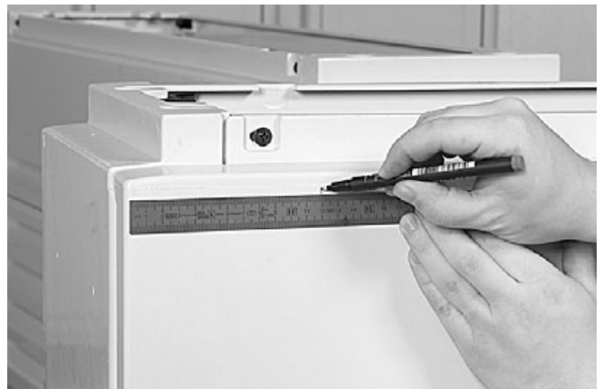
10.1.3 Mark at 120 mm starting from the side.
