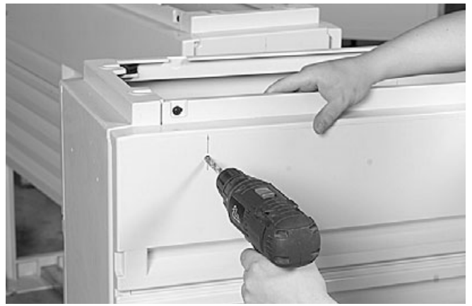
10.1.5 Drill the two holes ( \varnothing 8.5 mm).
