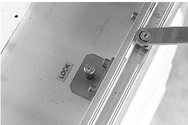
10.2.11 To lock the protection plate.
