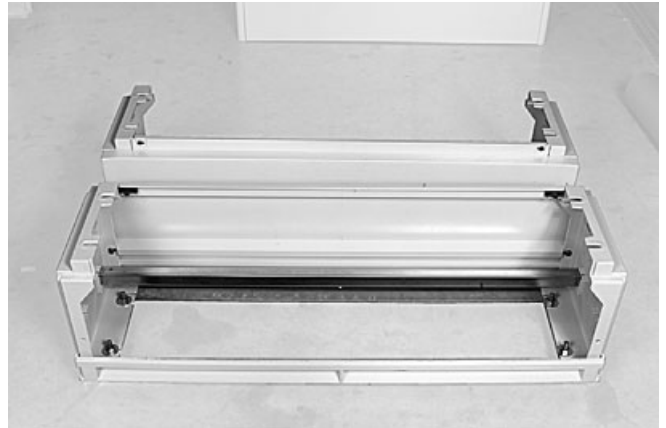
10.1.2 Fix the pedestals on the frames.
