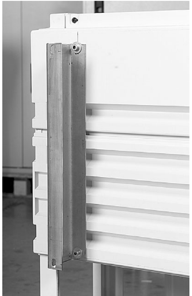
10.1.6 Install the connection kit and tighten the nuts (20-25 Nm).
