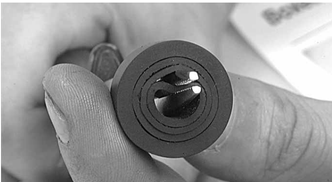
4.1.2. In case the cable diameter does not match with the diameter of the gland seal, remove the plastic nut, metal ring and rubber seal inside the gland and peel out some of the break out rubber rings up to the right diameter.
