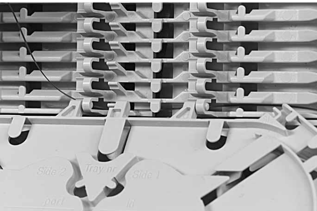
5.2.5 Route the fibers in the grooves of the wraparound groove plate to the entrance of the identified tray. Fiber must be routed in the groove underneath the tray hinge.
