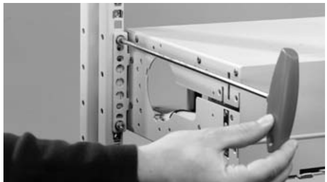
3.1.3 Mount the unit using the FACC-ALLEN-KEY.
