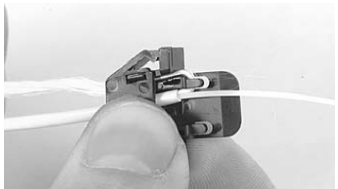
5.2.7 Slide the inner part to the left as much as possible by pulling the jacket and kevlar at the same time. Cut the excess kevlar leaving 5-10 mm.
