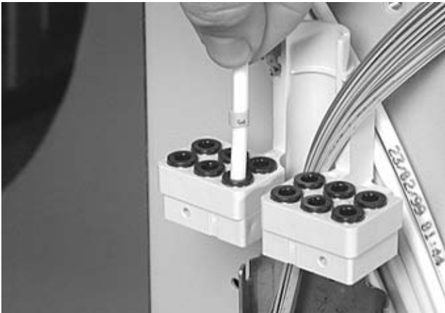
4.1.29 Insert the tubes in the connectors. Use 6 positions at the left when cable is mounted at the left side of the bracket.
