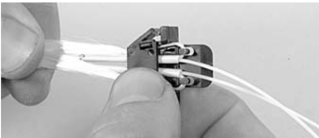
5.2.11 Slide the inner part to the left as much as possible by pulling the jacket and kevlar at the same time.
