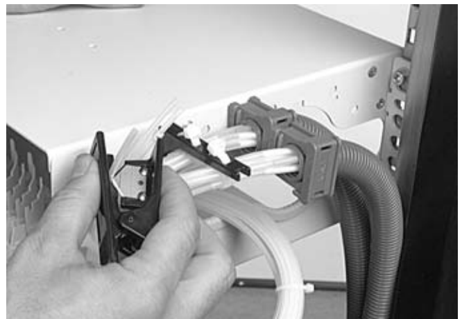
4.1.17 A second cable can be added by using the second flex tube holder.
