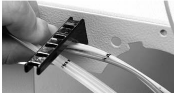
4.2.6 Mark the transportation tubes 10 mm from the plastic stand-off. Mark the loose tubes 30 mm from the plastic stand-off.
