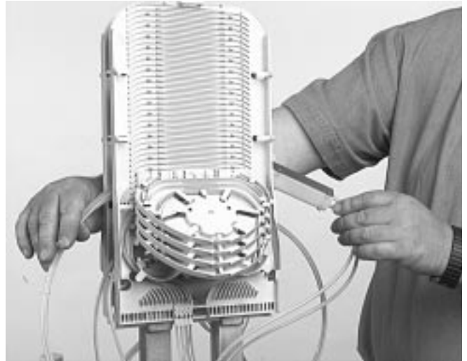
11.12 Bring the FOPT protection tubes together with tie wraps.
