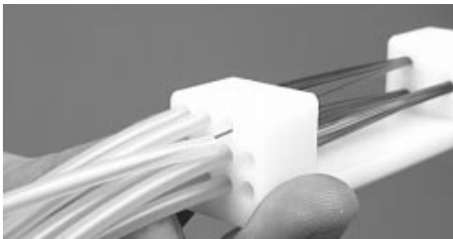
11.10 Cut the FOPT-CS to a length of 700 mm. feed the fibers through and push the FOPT-CS in the PECO 3/12 outlets. Pull gently on the fibers.
