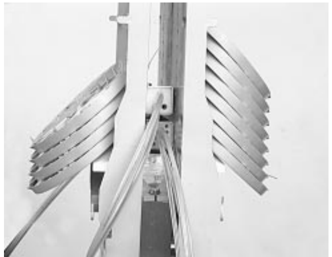
11.13 Position the PECO 3/12 between the two FAS plates. Be careful not to kink the FOPT protection tubes.
