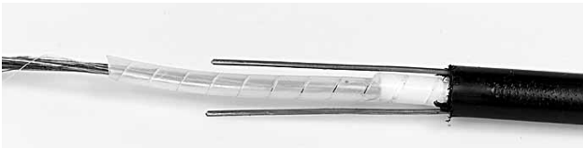
4.2.39 Put the spiral tube on the cable
