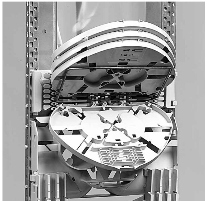
6.6 Identify the tray to be worked on and make it accessible. If the routing block and trays are in vertical position you will have to support the trays above the selected one using the tray wedge which fits in the cavities of the wraparound groove plate. Position the wedge carefully such that the groove is still accessible for the fibers and be careful not to push the wedge against fibers. To remove the wedge, use two hands to pull on both ends (near the groove plate).
