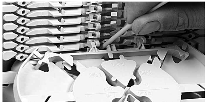
6.5 To remove the tray put the fiber guiding pin between lip on wraparound groove plate and tray and move lateral towards S1.
