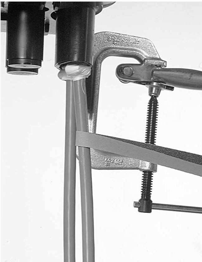
5.1.2 Clean and abrade the cable.
