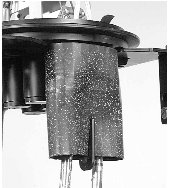
5.1.5 Push the sleeve against the base and place the clip.
