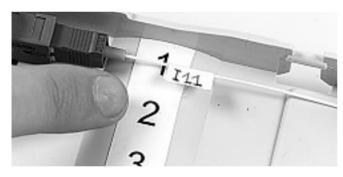
3.2 The identification (printed on the flags next to the connector boot) of the pre-assembled 900 micron pigtails is as follows
