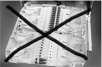
2.3 Make sure that the replaced tray and replacing tray have the same connector position.
