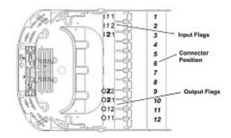
Example: component 1: 2x2 splitter; component 2: 1x2 splitter The drawing shows the connector positions and the flags identification
