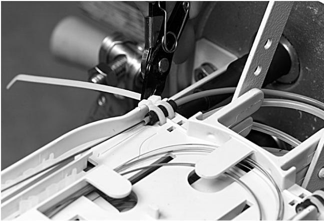
12.6 Route loose tube or FOPT-CS to appropriate tray and mark tube at 15 mm from edge of tray. Wrap foam around loose tube or FOPT-CS and strap it to the tray with two tie-wraps.
