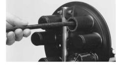
14.5 Align cable ring cut with the edge of the base. Slide strength member into clamp and tighten the nut. Cut away the excess length of strength member.
