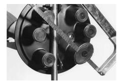
4.3 Remove any dirt, mud or other contaminants from the cable sheath for approximately 2 meters with a clean cloth. Take the oval cable seal and slide it over the cables. The non-coated edge of the sleeve and the arrows should be pointed to the base of the closure.
