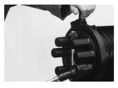
13.2 Remove carefully the dome and the sealing ring. Keep the sealing ring and seal area of the closure free of dirt. (If needed rinse with clear water).
