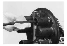
14.7 Abrade port and cable sheath circumferentially on the cleaned area with the abrasive strip. Remove any abraded material with a clean cloth.
