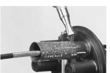
14.11 Shrink down the end of the sleeve on the cable side. Heat till the sleeve shrinks down onto the cable and the green thermo-indicating paint is converted to black. A ring of red adhesive should be visible at the cable on the end of the sleeve.
